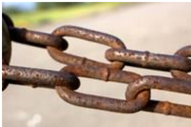
The iron in these steel chains has started to rust.
