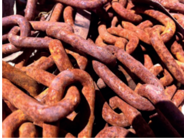
The iron in these steel chains has started to rust.
